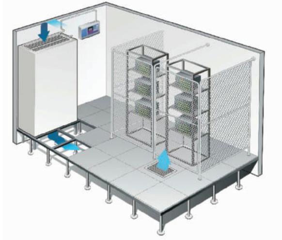
Illustration 2: Smoke detection at the CRAC return air grille.
